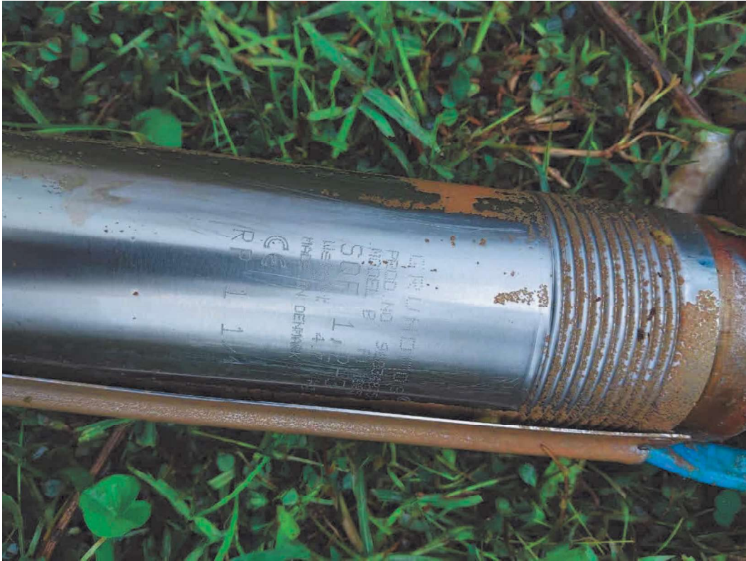
Figure 6: The faulty Grundfos SQF 1.2-3 submersible pump with traces of silt on the outlet
